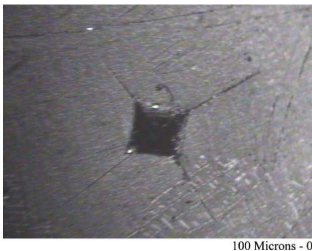
Fig. 6 Representative indentation of glass-ceramic 4-21 with resultant crack lines
